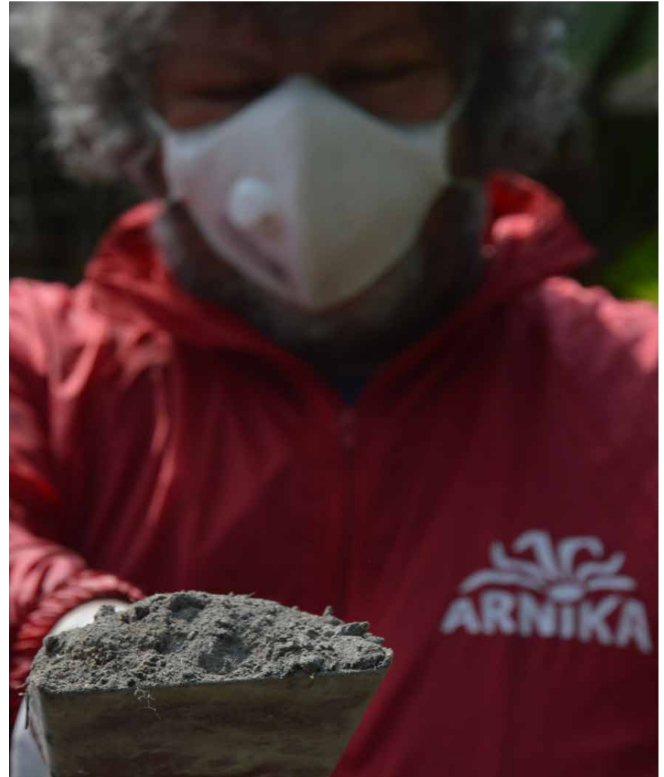
Photos 4.33 – 4.35: A small abandoned medical waste incinerator near a hospital in Accra, Ghana. A pile of ash residues from waste incineration showed relatively high concentrations of dioxins. Leaving it accessible to chickens resulted in elevated levels of dioxins in their eggs. Analyses of samples taken by Arnika in 2018 confirmed this hypothesis (Hogarh et al. 2019; Petrlik et al. 2019a). Photo: Martin Holzknrecht, Arnika
