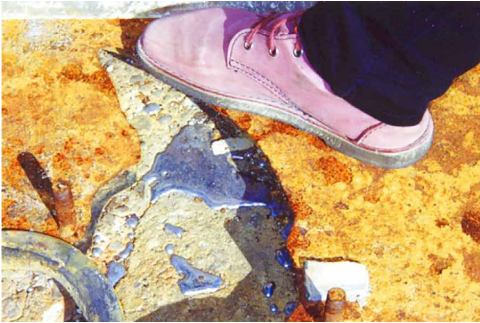
Photos 3.4 and 3.5: Mercury is especially ubiquitous in old chlor-alkali plants (Mach et al. 2016; Mach et al. 2023). In photograph 3.4, mercury contamination is shown in the bombed Pancevo plant in Serbia in 1999 (photo 3.5) (Associated Press 2010; UNEP and UNCHS 1999). PRTR helps to keep records of mercury flows. Photos: UNEP archive
