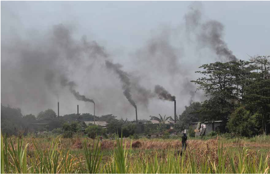
Photos 5.4 - 5.5: Tofu factories in Tropodo replaced wood with plastic waste as fuel and became a serious threat to public health. High levels of POPs, including dioxins and/or BFRs, were measured in local food sources (Ismawati et al. 2021; Petrlik et al. 2019b). Such pollution sources should be somehow included in future PRTR in Indonesia. Photo: Jindřich Petrlik, Arnika, 2019
